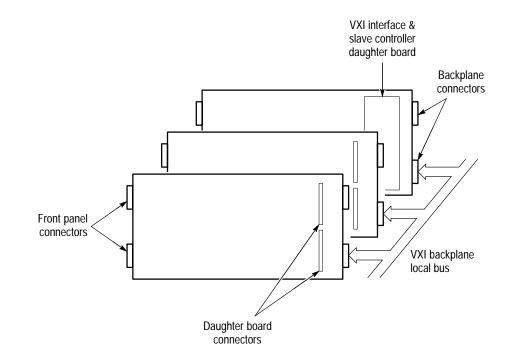
Figure 1–2: Typical SurePath Configuration
